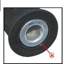
Throttle Sleeve (when bar-end is removed)
